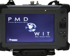
The Astronics DME Wire Integrity Tester (WIT) is a portable, self-contained test platform used for verification testing and fault detection, isolation and repair of metallic wiring. The tester contains the hardware and software necessary to test and verify the integrity of wiring in a field deployed, depot, or factory type environment.
