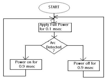
Figure 7 – Control Algorithm Assuming Perfect Knowledge of Arc
