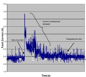
Figure 8 – Fault Current to a Carbonized Parallel Path Under Control (Note that the current scale is different than that of Figure 6)
