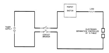
Figure 2 --- Test Bed Schematic for Series Arcing Experiments
