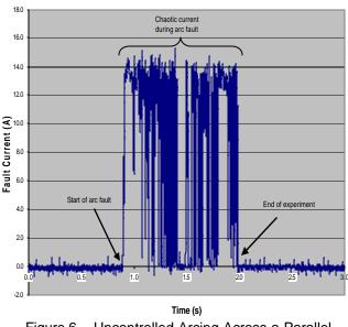
Figure 6 – Uncontrolled Arcing Across a Parallel Carbonized Path
