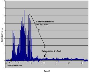
Figure 10 – Fault Current Under Adaptive Control and Assuming Realistic Delays
