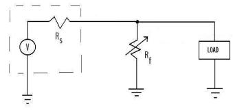
Figure 12 – The Parallel Arcing Case
