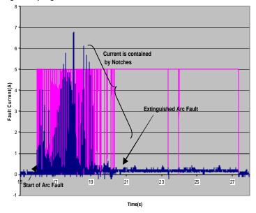
Figure 11 – Fault Current and Gate Signals for Adaptive Control
