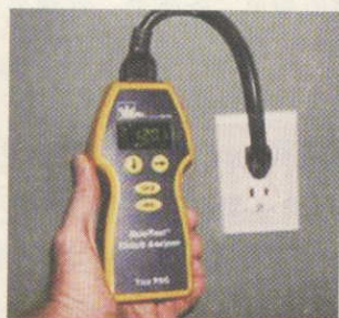
图7 AFCI现场验证仪表与故障模拟信号 Fig. 7 AFCI instrument for on-site verification instrument and analog fault signal
