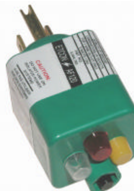
Figure 7 – ETCON "AFCI" Tester →
